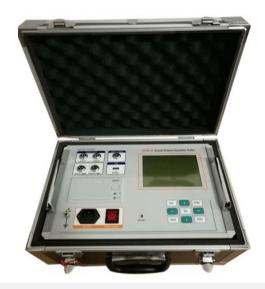
This High voltage switch mechanical characteristic test instrument can be used to test and measure mechanical parameters of vacuum, sulphur hexafluoride, less oil, more oil power system's high voltage switch and etc. It is the most convenient tool for high voltage switch's repairement and test for its stable data of measurement, easy wiring and simple operation.
